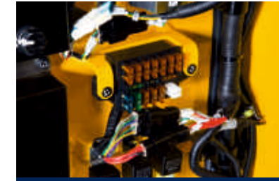
Centralized fuse box
