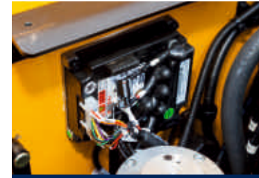
Reliable MOSFET type controller
